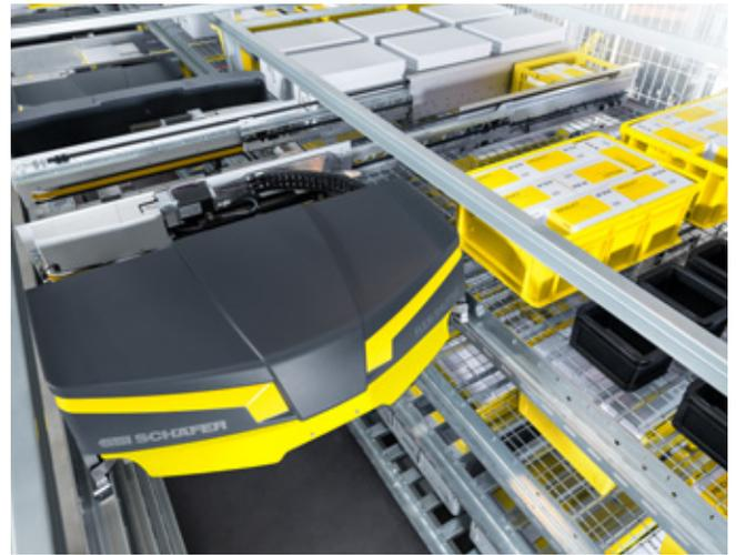
High-density tub and carton storage provided by an AS/RS system allows for sufficient quantity of stored units during peak periods.
