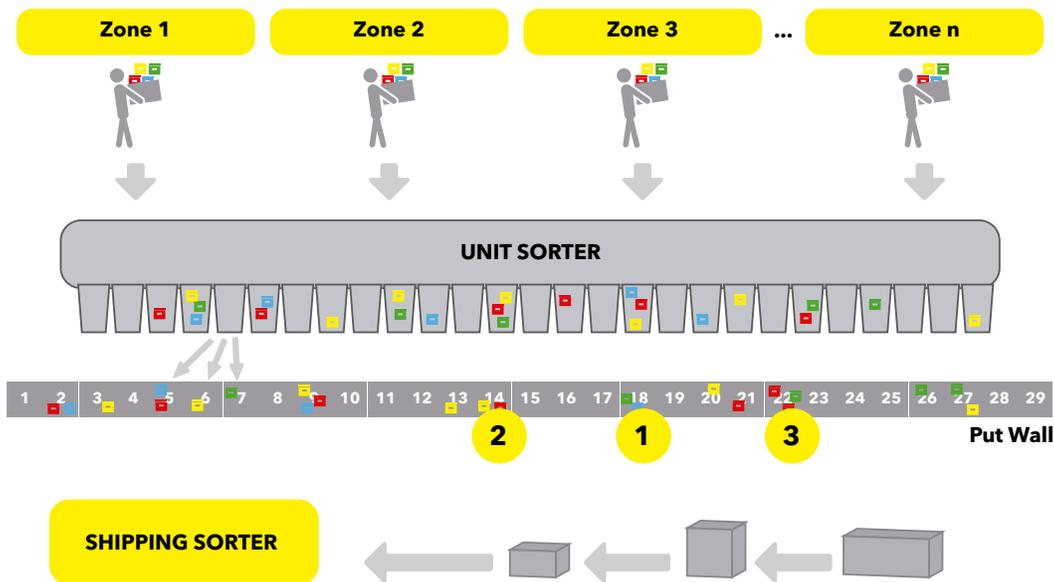
The number of sort/put destinations limit the batch size. This limitation produces a low pick density, unproductive picking, and a large labor force. Inefficiencies compound when large labor forces get too far out of sync and orders cannot be cleared.
